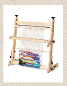
Weaving on a loom is done by intersecting the longitudinal threads, the warp threads (threads that are thrown across), with the transverse threads, the threads (threads that are woven). The major parts of a loom are the warp and takeup roll.
